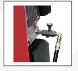
Even though all cylinders are flow restricted inside, we are adding the flow controlled valve to control the lowing speed for the heavy-duty line four post lifts model R4P-14K and R4P-14KA
