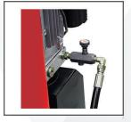
Even though all cylinders are flow restricted inside, we are adding the flow controlled valve to control the lowing speed for the heavy-duty line four post lifts model R4P-9K and R4P-9KA
